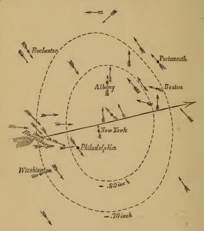
which the barometer sunk eight tenths of an inch below the mean, and the larger oval shows the area within which the barometer was depressed seven tenths of an inch. The long arrow represents the direction in which the storm advanced, while the short arrows show the observed direction of the wind at nearly forty different stations.
